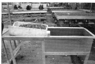
Total Immerse tank at a Dutch ivy rooting station. The dip basket is not shown.
